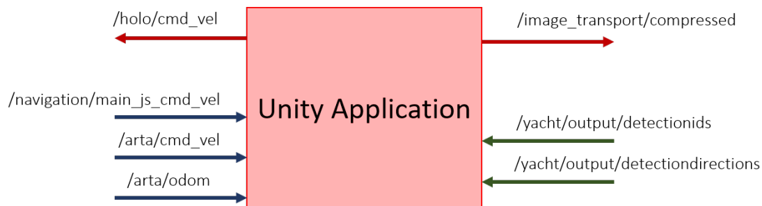
Figure 5.16: ROS topics in and out of the Unity application. Each topic carries data used by different parts of the overall system.
