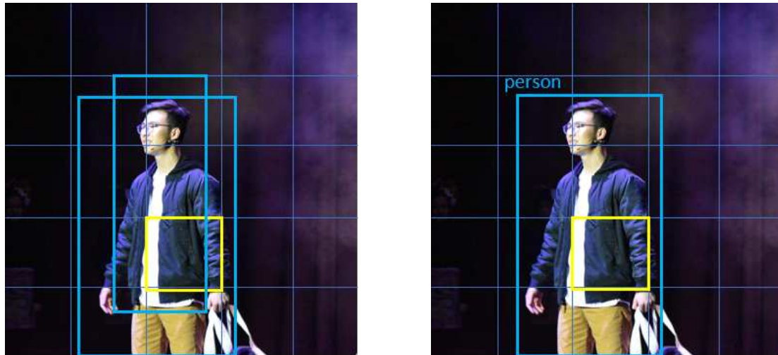
(a) A grid cell can make B predictions, in this example B = 2 .
