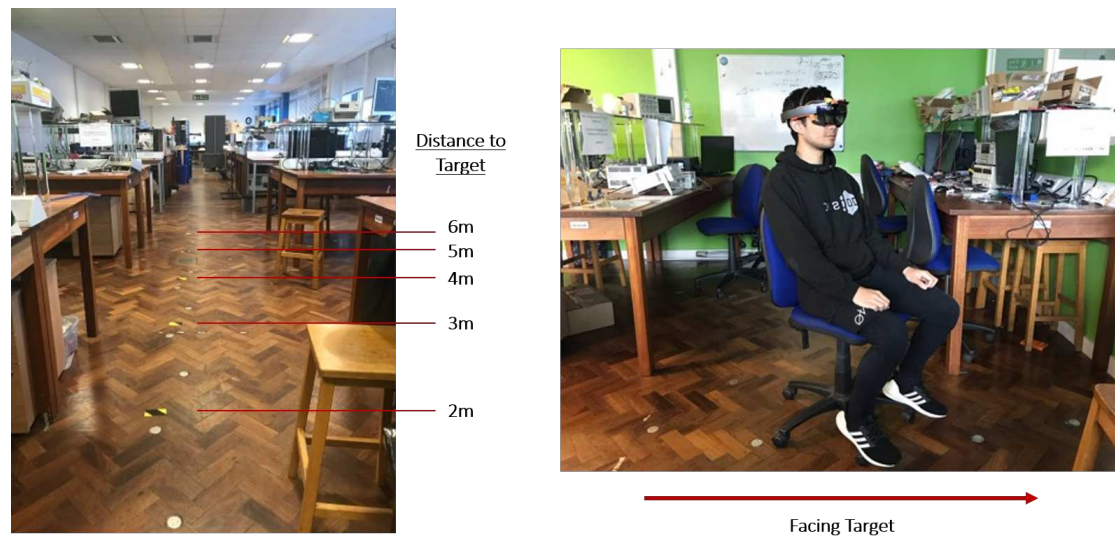
Figure 6.1: The experimental setup used to test the HDD and Hololens spatial mapping accuracy. We asked the people acting as targets to stand at 1 meter intervals while a person sitting down wearing the Hololens looked at them using the front facing camera.
