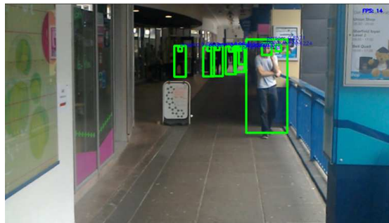
Figure 5.5: Trained model detects people and heads at different ranges. We also see it can detect people far away and accurately detect their heads.
